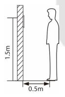
The distance between the device and a user whose height is within 1.4m-1.8m is recommended to be 0.5m. Users may slightly move forwards and backwards to improve the quality of facial images captured.
